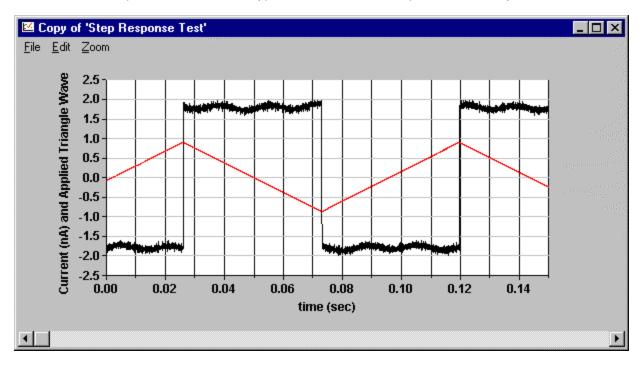
However, the 428 has some very flexible filtering options as the next graph shows. In this case, the applied signal is unchanged, but the programmable rise time filter feature was turned on. A rise time of 1 msec was used. As can be seen, the noise is reduced but at the expense of response time. Even so, these data clearly demonstrate the superior response time of the 428 current amplifier for situations where measurement of a rapidly changing signal is the primary goal.
