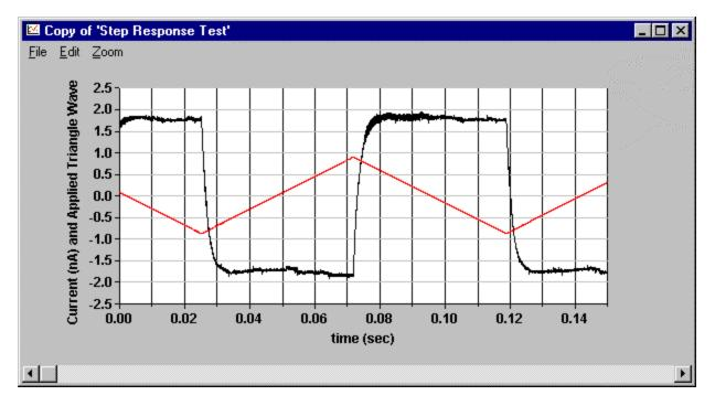
Below are data from a model 6485 picoammeter. The picoammeter was on the 2nA range; filtering was OFF. As the graph demonstrates, similar to the results with the 6487, there is a significant response time. The response time of the 6485 is longer than for the 6487.
